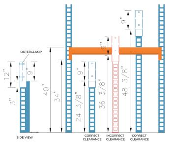
This illustration shows how to avoid interference issues with beam end plates and other attachments. The area of the outer clamp prohibits re-connection.
